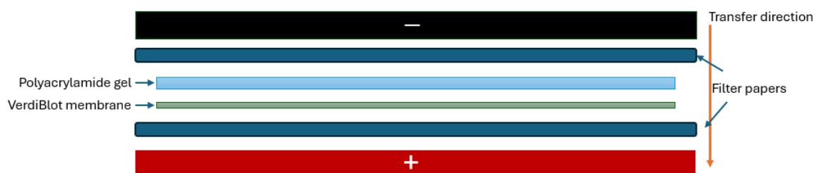
Fig. 1 In the schematic, note the order of components cathode to anode: sponge → filter paper → gel → VerdiBlot membrane → filter paper → sponge. Ensure the membrane faces the positive electrode (anode) to drive negatively charged proteins out of the gel onto the membrane.
